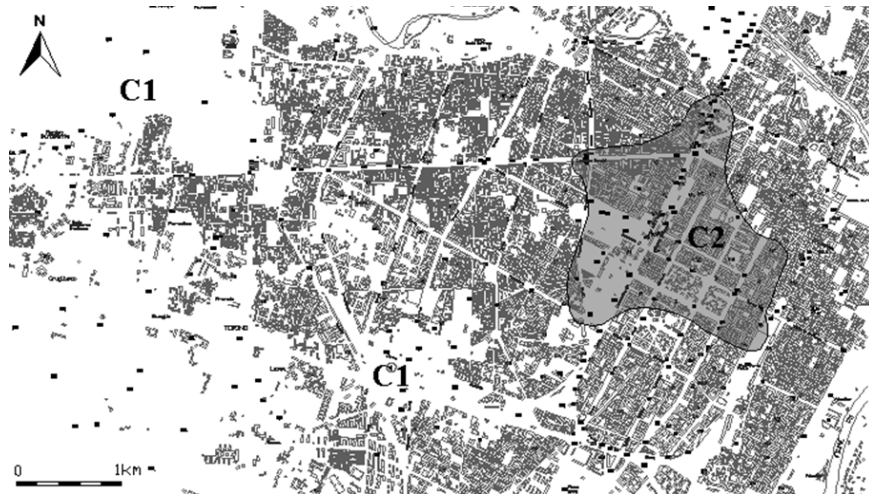
Fig. 2. Map of the cementation degree in the subsoil of Turin (10 m below the surface) (from De Rienzo and Oreste, 2011): C1: not cemented layers; C2: cemented layers; red circle: location of the realized diagraphies, on the border of the area C2
