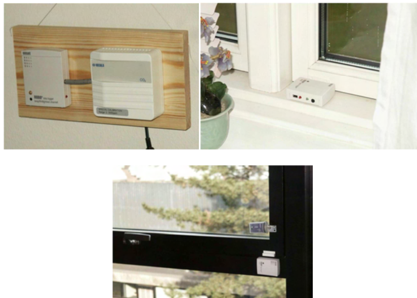
Figure 2. Pictures of the instruments used to measure the indoor environmental variables and window opening behaviour. Top left: CO 2 monitor connected to a data-logger with built in temperature, relative humidity and illumination sensors. Top right: Window state sensor (open/closed). Bottom: window state sensor (open/closed) and window position sensor.
