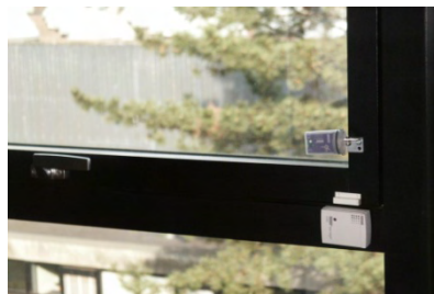
140 Figure 1. Pictures of the instruments used to measure the indoor environmental variables and window opening 141 behaviour. Top left: CO 2 monitor connected to a data-logger with built in temperature, relative humidity and 142 illumination sensors. Top right: Window state sensor (open/closed). Bottom: window state sensor (open/closed) and 143 window position sensor.
