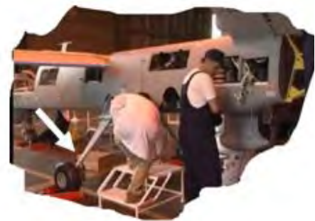
Figure 18. example of tapered leaf spring landing gear
