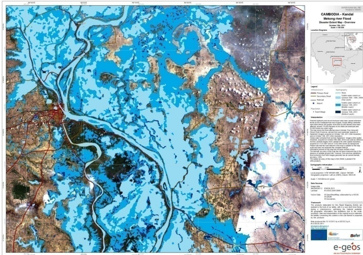
Figure 1.1 Map produced by the SAFER project after an activation with focus on floods in Cambodia. The map shows the flooded areas extracted from the classification of satellite imagery in two different days after the events, in comparison with the normal conditions of a pre-event satellite image; the base reference data is constituted by a satellite image in true colours and vector sources of transportation network and settlements (source SAFER website).
