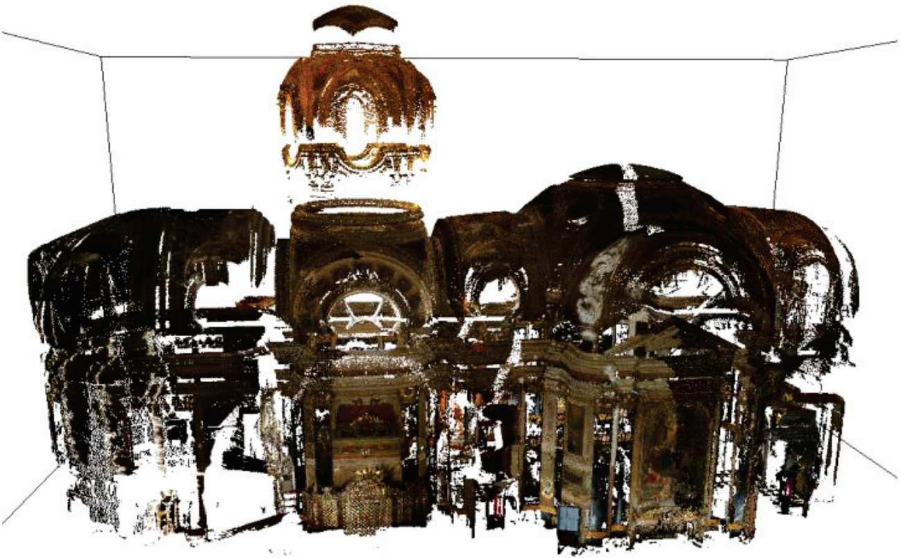
Fig. 7 - Point cloud images created by the laser scanner
