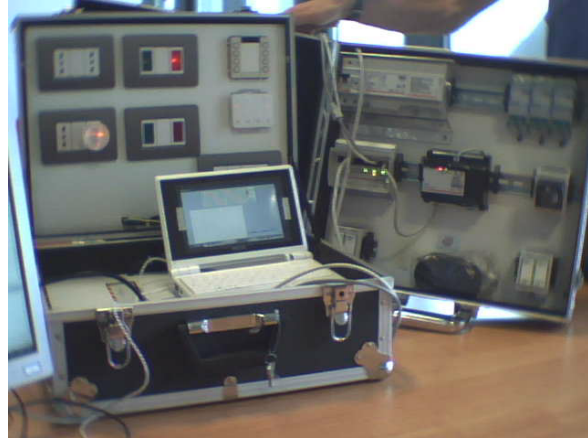
Figure 13: The demo cases used for the emulation of the Bank Security Booth use case, and the Asus eeePC running DOG.
