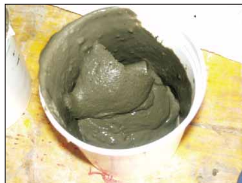
Figure 5. Grout mix after hardening.
