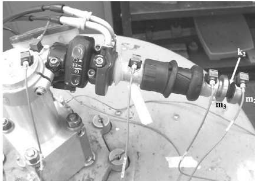
Fig. 9 The handle with the proposed vibration absorber
