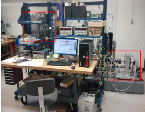
Figure 7. View of the test rig. The dSPACE 1103 PPC host computer is on the desk. The machine-under-test is in the red square to the right, connected to an induction machine dynamometer via an inline torque meter (not visible). The red square to the left identifies the power converters.
