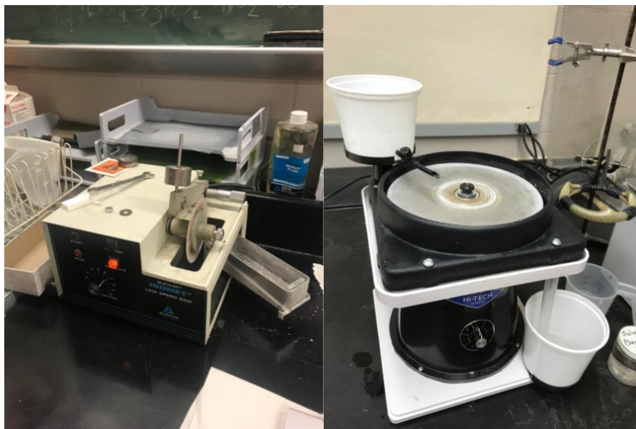
Figure 3: On the left shows the saw that was used to cut the spinel samples. On the right shows the polishing wheel. This machinery was used at Augustana College in Rock Island, Illinois.
