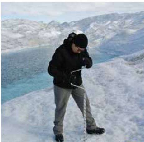
Left: Rutgers graduate student Samiah Moustafa on the Greenland ice sheet drilling a hole used to install an ablation stake to measure melt rate. Photo: Åsa Rennermalm ; Right: Rutgers representatives working at the U.S. Naval Arctic Research Laboratory at Point Barrow, Alaska in 1957. Left to right: Professor John Tedrow, William Gillis '55, Professor Russell Alderfer, John Cantlon '50, James Drew '52, Nathan Perselay '23, graduate student Lowell Douglass, Jerry Brown '58—and Ambercrombie, the mascot. Photo: Jerry Brown
