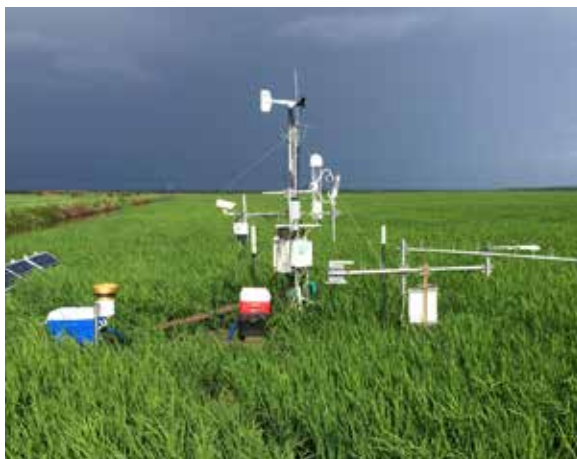
Left: Meteorological measurement station in a rice field in central Arkansas after a summer storm (2015). Right: The icebergs left by the flood of the Lena River in 2014. Photos: Benjamin Runkle
