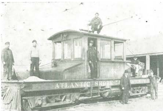
NO. 102 as it was originally built. When locomotive 101 was rebuilt to an express car, its cab was added to No. 102. —Photo from the collection of Howard T. Moulton.
