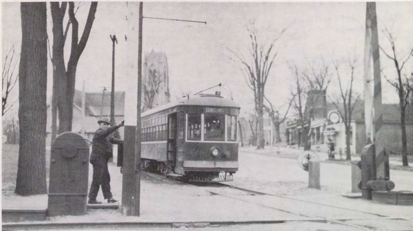
THE ONLY steam railroad grade crossing on the Lewiston-Bath line was on Maine Street, Brunswick, where the trolley crossed the main line of the Maine Central. Here is No. 120 waiting for the crossing tender's signal to go.
