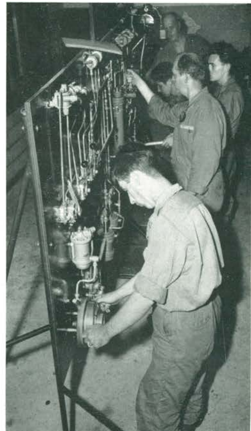
Douglas Hydraulic System Mockup.
