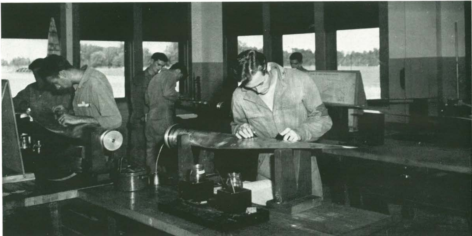
PROPELLER INSPECTION AND REPAIR
