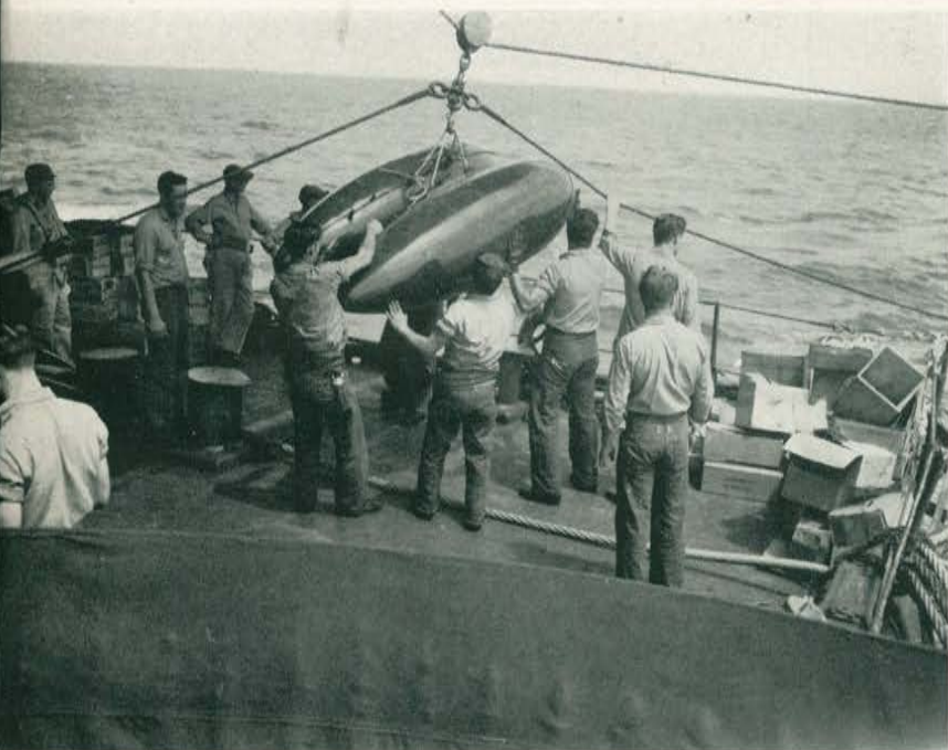
Returning empty belly tanks by the whip (a form of breeches buoy).
