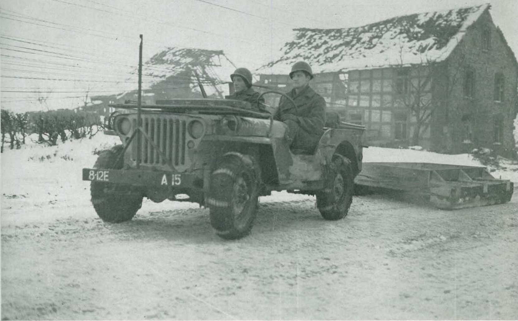
This sled which is attached to the jeep will be used to haul ammunition to their unit over snowy roads
