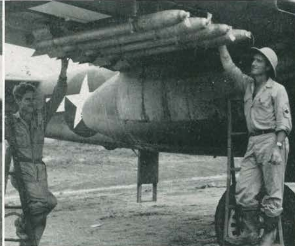
The rocket installation shown here was the last wartime addition to the Mitchell's punch. These, plus 14 calibre .50's and a ton of bombs, made the B-25 an outstanding ground support weapon.
