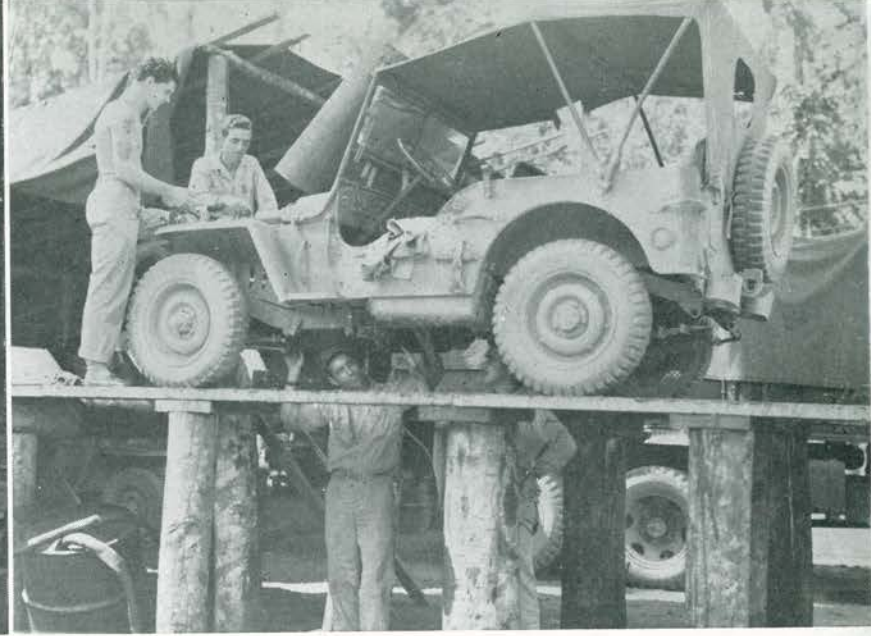
The grease rack at your corner filing station is probably prettier, but Transportation in New Guinea kept them rolling with a rack like this.
