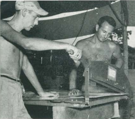
A couple of proud inventors demonstrate the sheet metal cutter they devised from some old armor plate, a spring, and a few nuts and bolts. Very superior to shears.
