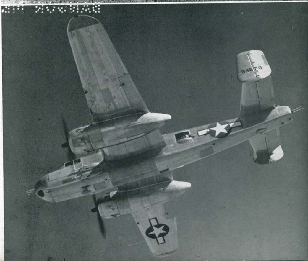
Old "Pistol Packin' Mama," the H, incorporated the improved 75-mm. aircraft cannon. Tested thoroughly, they were found a little unsuitable for our type of operations.
