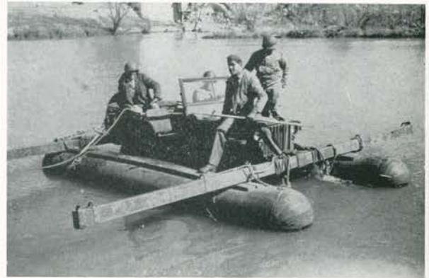
Top: Sequin, Texas, near Fort Sam Houston. Improved jeep floats for river crossing.
