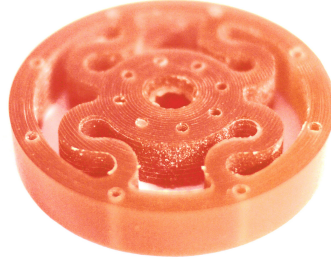
Fig. 7: Manufactured polyurethane-based torsional spring.
