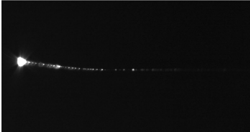
Figure 2.13: Characteristic pearl-necklace pattern resulting from contamination of an ONF by particles. No more than 1 \mu\text{W} of power was launched into the fiber to take this picture. Increasing the power beyond this point broke it.
