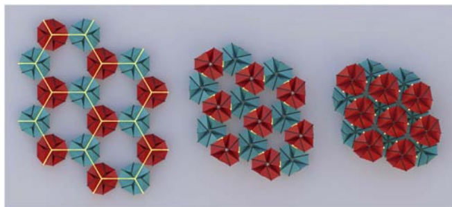
Fig. 7. Rendering of a deployable structure made from nine-hinged Möbius kaleidocycles (MK9). Each MK9 is connected through extended hinges (yellow) to three other MK9 with opposite chirality (distinguished with red and blue) to form a hexagonal lattice. If the MK9 performs the everting motion, a contraction from the extended state ( Left ) to a contracted state ( Center and Right ) occurs.
