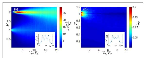
**Figure 10.** Standard deviation of (a) the average momentum and (b) the time-averaged coherence as a function of the lattice depth and the filling ratio. The insets shows the same near F = 1 for a lattice depth of  $V_0 = 0.1E_r$ . These plots are based on calculations for M = 50 and with the time-average taken over the interval 0 to  $10t_0$ .
