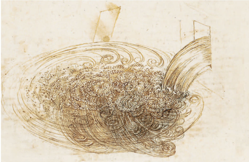
Fig. 1.1: Leonardo da Vinci’s sketch of a turbulent flow (chalked on paper, dated A.D. 1494). This turbulent flow consists of what might be termed as a “turbulent cauldron” that forms where a water jet, discharged from an orifice in the vertical wall on the right side of the sketch, plunges into a large pool of still water. The turbulent cauldron contains myriad eddies in a broad range of sizes; the largest eddy encompasses the entire domain of the turbulent cauldron whereas the smallest ones, which are quite numerous, have a characteristic size that is but a minute fraction of the size of the turbulent cauldron. The presence of eddies in a broad range of sizes is a cardinal property of turbulent flows (Sreenivasan, 1999; Davidson, 2004).
