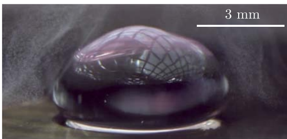
FIG. 4. Acetone droplet ( D \approx 6 mm) in a Leidenfrost state hovering on a polished copper substrate with a temperature of \approx 200 °C. The picture comes from a sequence of images obtained at 2500 FPS. An aerosol which is made from small water droplets surrounds the acetone droplet. The reflected pattern on the surface of the droplet is from a basket containing the dry ice which is used to generate the aerosol. (Multimedia view) [URL: http://dx.doi.org/10.1063/1.4977442.3 ]
