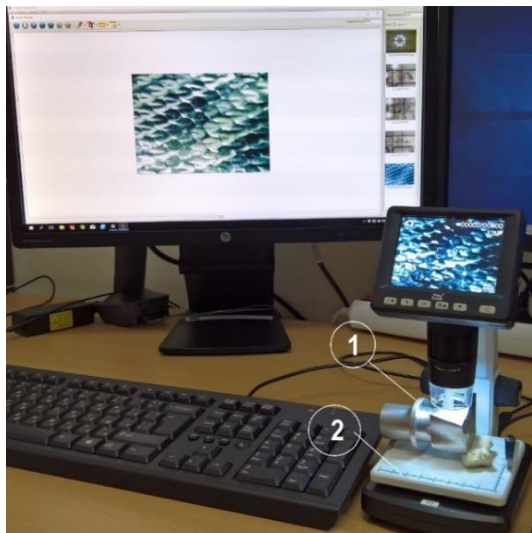
Fig. 2. Digital microscope DigiLab5.0+, connected to a computer to obtain RR images of high resolution
