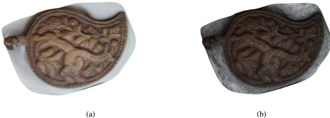
Fig. 8. Model 2 - Digital model of a belt-buckle in Autodesk ReCAP environment: (a) with texture; (b) with wireframe and texture.
