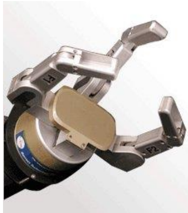
Figure 2.4: Barrett hand. (Source: Robotiq.com)
