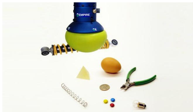
Figure 2.12: Universal gripper handling different shaped objects. (Source: GRABCAD)
