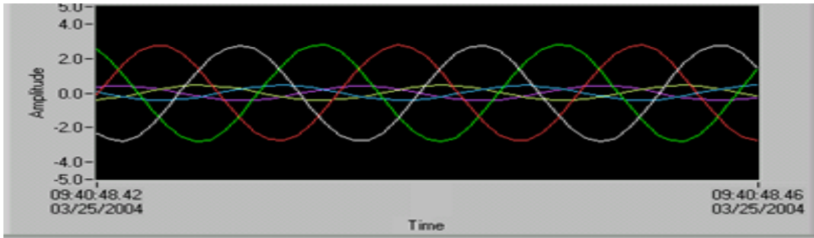
Figure 4.8. Under Voltage Fault.
