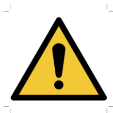
Figure 9. This image is an example of an ISO warning sign meaning “general warning.” Copyright International Organization for Standardization.
