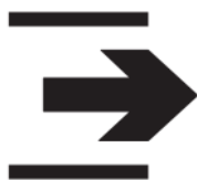
Figure 16. This ISO graphical symbol is labeled “way out or exit” and shows a right-pointing arrow contained between two parallel lines. It is an example of a symbolic graphical symbol because an arrow is an abstract concept. Copyright International Organization for Standardization.
