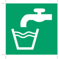
Figure 12. This image is an example of an ISO safe condition sign meaning “drinking water.” Copyright International Organization for Standardization.
