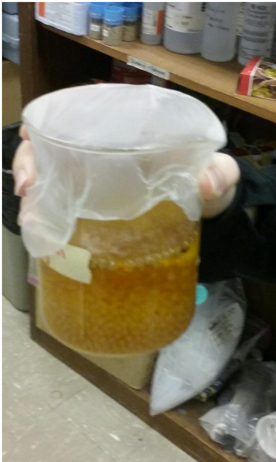
Figure 5. The polymer beads after they were made by dropping alginate in a \text{FeCl}_3 solution.
