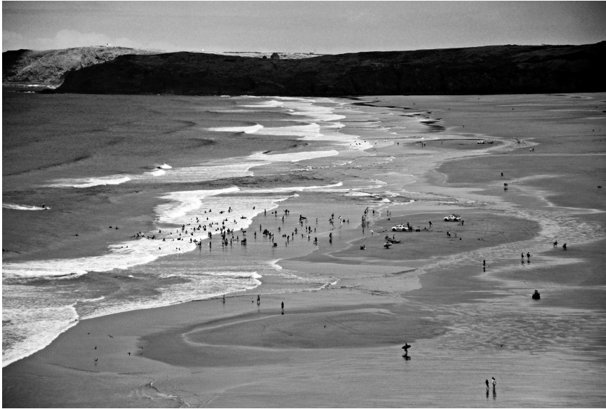
Figure 1 — Image of low-tide Perranporth Beach, UK, showing multiple sand bars and rip currents, lifeguard flag placement, and location of bathers (photo used courtesy of Tim Scott).
