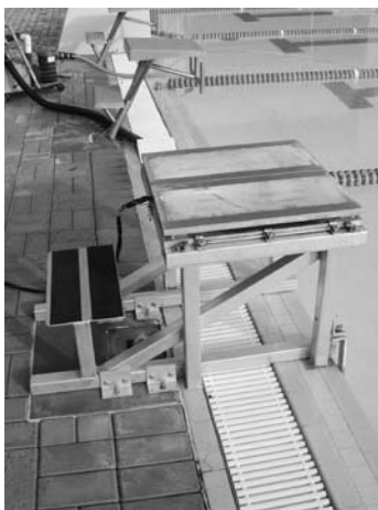
Figure 2 — The starting block with the force plates mounted.
