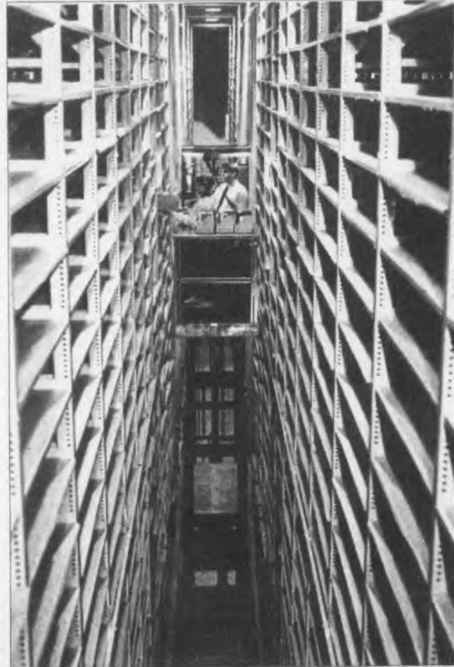
Student workers use a modified fork lift, nicknamed "Eleanor," to shelve and retrieve stored library materials at the Northwest Ohio Regional Book Depository.
