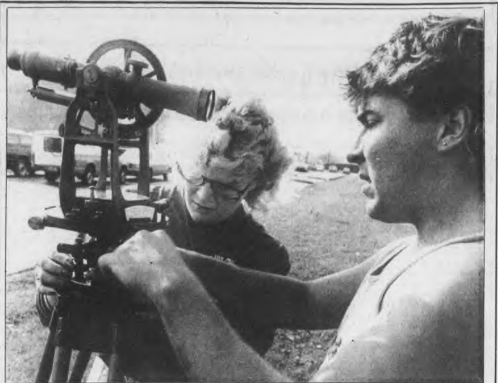
Class Survey Junior Pamela Pinchot and senior Chet Laquatra adjust a surveyor's transit near the Technology Building Thursday afternoon. The two were working on a project for their Surveying 318 class, in which they were required to survey and draw a topographical map of a field behind the Technology Building. BG News/John Potter
