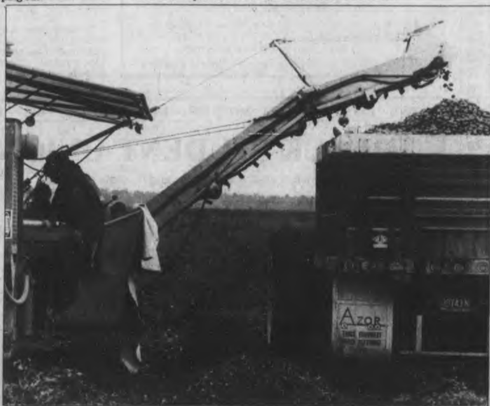
After this automated tomato harvester cuts the vines and brings the tomatoes to the platform, the workers shake the dirt off and remove the remaining vines.
