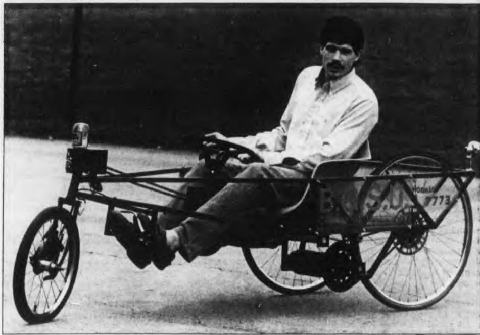
Derek Paetow, junior industrial technology education major, drives the spring-driven car which won first place in the Olympics of the Mind Collegiate World Finals. Paetow also helped build the car for the competition.
