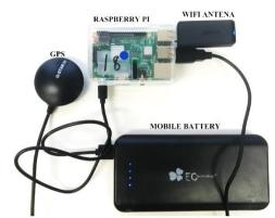
Figure 3. WiFi Scanner, GPS and Mobile Battery Source: Transport Laboratory TUS Asset
