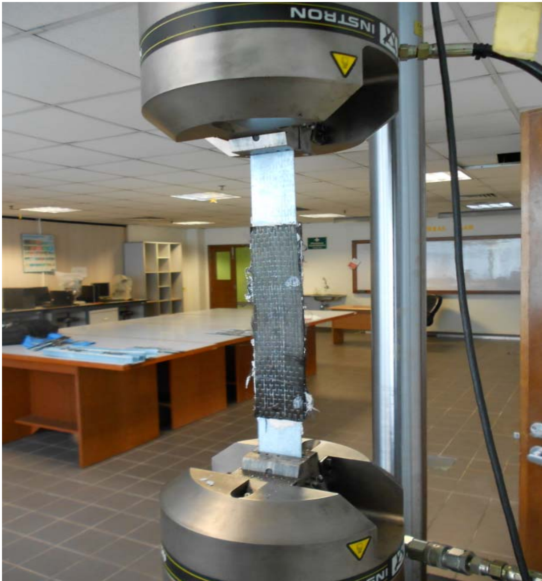
Figure (1): Tension coupon test with CFRP strengthened specimen
