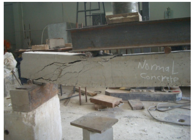
Figure 3: Failure of the control beam
