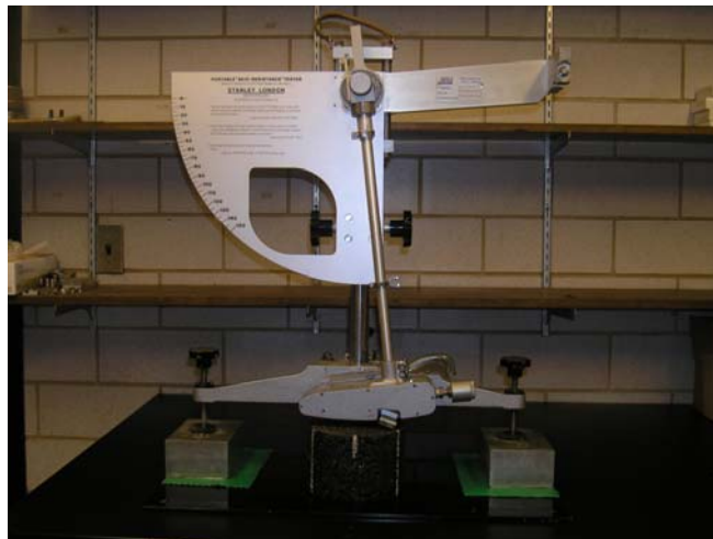
Figure 2: Friction measurement setup using the BPT
