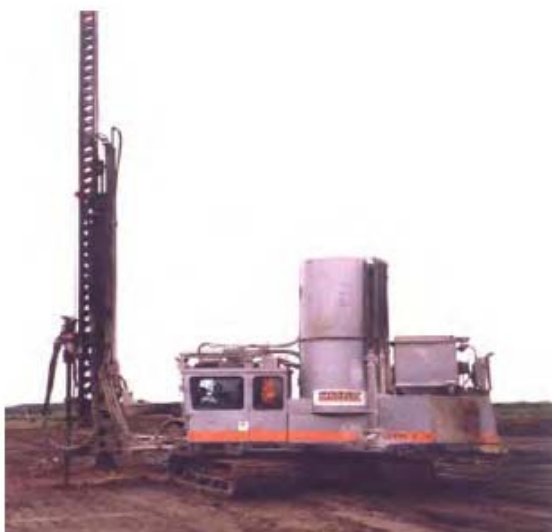
Figure 2: (a) Deep wet mixing plant; with (b) separate mixing and holding tanks and pumps
