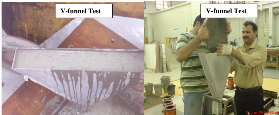
Figure 2: V-funnel test for evaluation of segregation resistance
