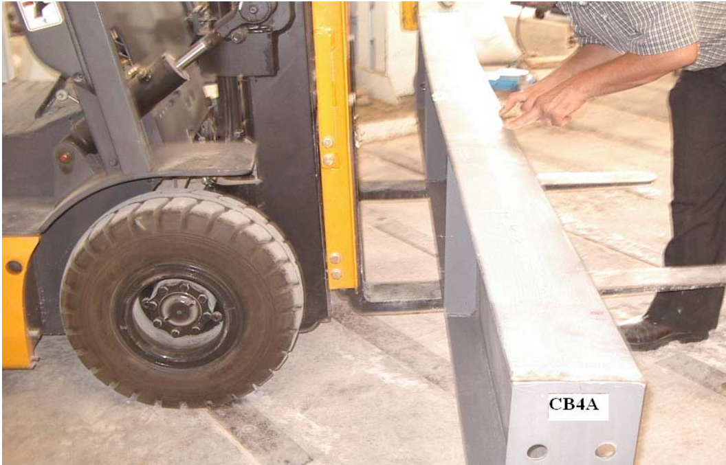
Figure (11): Lateral-Torsional Buckling Mode in Beam CB4A.
