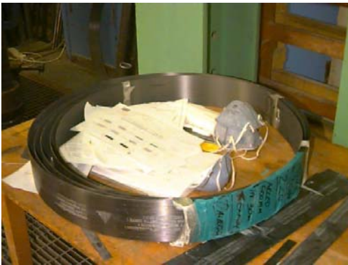
Figure (1): Pultruded Carbon Fibres.
