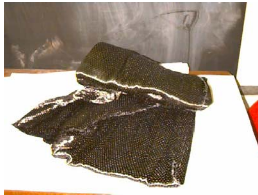
Figure (2): Prepreg Carbon Fibre.
