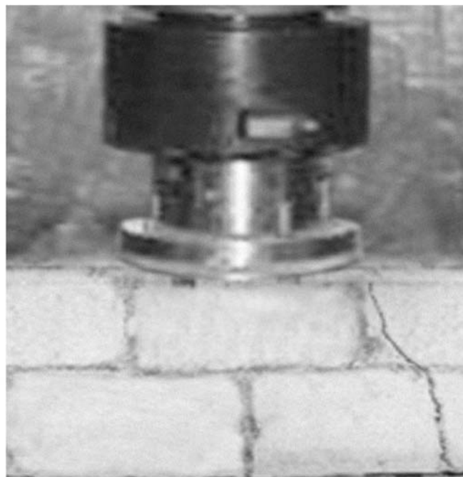
Figure (3): Shear Failure for Beam Tests.
