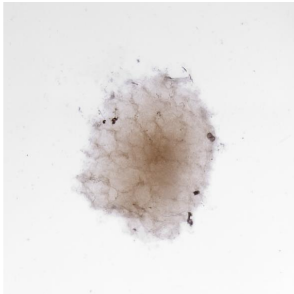
Figure 7. An organized structure in water sample subjected to temperatures up to 100 °C in the electric field of high voltage and and frequency. The material of the electrode – hostafan; electric voltage - 15 kV, electric impulse duration 10 \mu s; electric current frequency 15 kHz.
