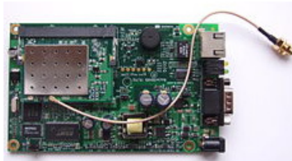
Figure 4: Wireless Card connected to router board
