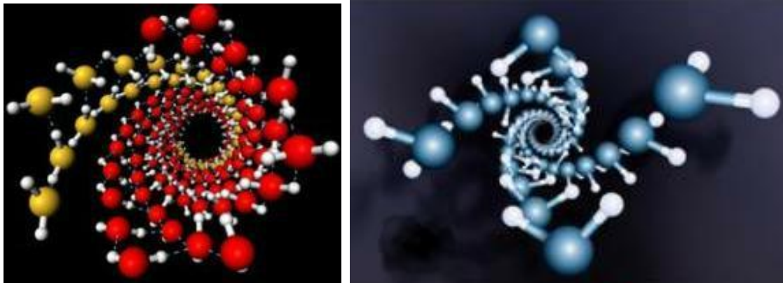
Figure 3. Structures of water crystals in carbon nanotubes according to computer simulations (Bai et al. , 2006) (diameter of nanotubes 1.35–1.90 nm; pressure 10–40000 atm; temperature -23 °C): a) – a general view of the crystal structure of water in nanotubes, b) – the inner wall of the structure of water.
