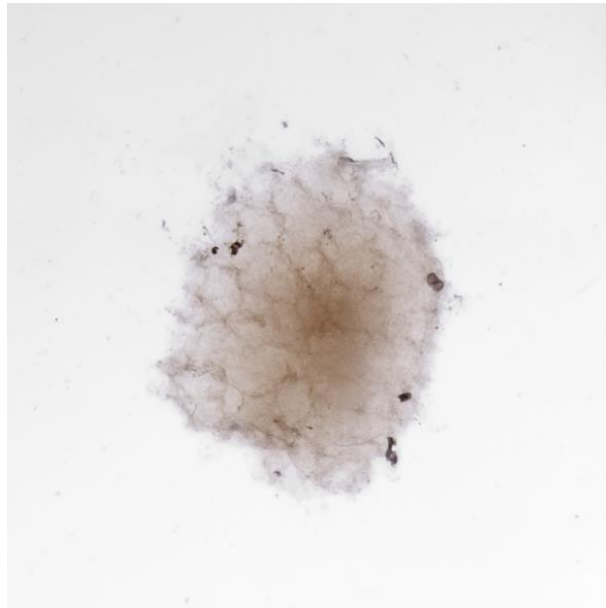
Figure 7. An organized structure in water sample subjected to temperatures up to 100 °C in the electric field of high voltage and and frequency. The material of the electrode – hostafan; electric voltage - 15 kV, electric impulse duration 10 µs; electric current frequency 15 kHz.
