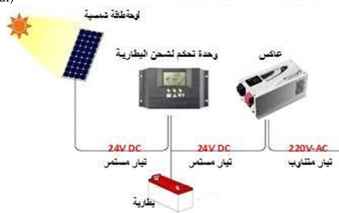
Figure. 2: Simple DC solar system
